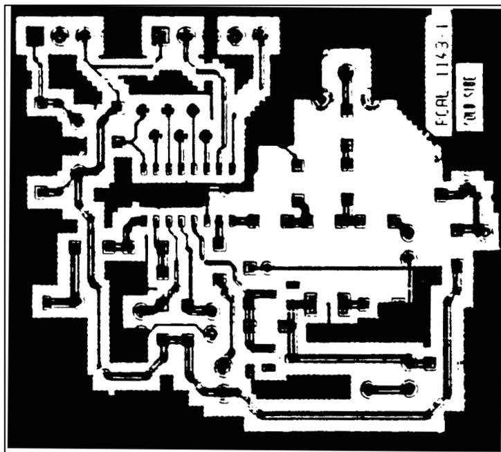
Figure 7. Board Layout for UMA1014T Frequency Synthesizer
