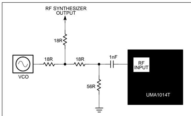
Figure 4. RF Power Splitter Circuit Diagram
