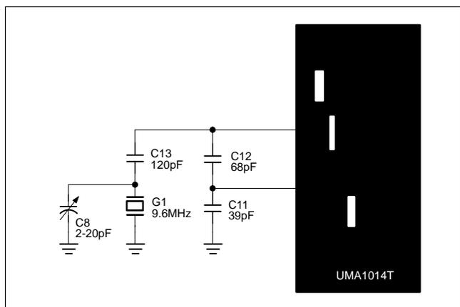
Figure 3. Crystal Oscillator Circuit Diagram
