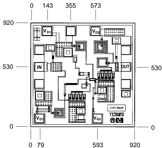
Figure 9. HMMC-5618 Bonding Pad Positions. (Dimensions are in micrometers.)
